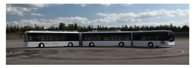
Scientists at the Fraunhofer Institute for Transportation and Infrastructure Systems IVI took up the challenge to make extra-long vehicles maneuverable in city traffic. This was achieved by equipping the vehicle with four steered axles in addition to the fixed main drive axle. A multi-axle steering system, developed and tested at the Fraunhofer IVI, has been implemented in the AutoTram® Extra Grand for the first time.
